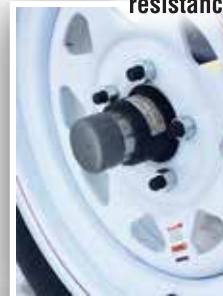
Wheels Spring loaded grease cups for water contaminate resistance.
